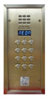
The Neon door panel range features marine grade 316 stainless steel fascias and back-box bezel. The back-box is galvanised and fixings are high quality tamper-proof torx (TX25) stainless machine screws.
